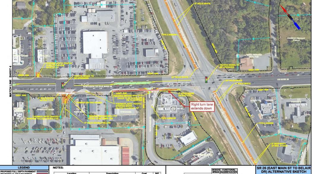
PROPOSED FULL DEPTH PAVEMENT I PROPOSED CLASS B PAVEMENT I PROPOSED MILL/OVERLAY CONSTR. I PROPOSED SIDEWALK PROPOSED MEDIAN / CAG PROPOSED MOUNTABLE MEDIAN PROPOSED LANDSCAPING/GRASS ANTICIPATED DISPLACEMENT ANTICIPATED DISPLACEMENT REMOVE EXISTING PAVEMENT & GRADE TO DRAIN PROPERTY AND EXISTING R/W LINE REQUIRED RW LINE
