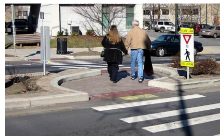
Figure 6.G.2 Pedestrian Crossing Island
